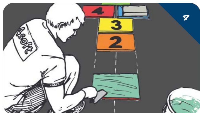
Spread the glue evenly on the underside of your graphic.
