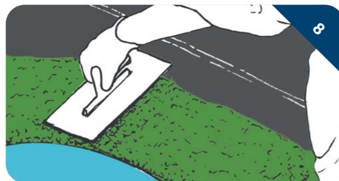
Spread and compress your final EPDM layer properly around the component.
